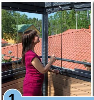
Push aside the pull knob in the bottom edge of the first panel. Pull at the string hanging from the upper latch and open the pane allowing it face the sidewall of the balcony. You may also leave the pane in the airing posi-tion if you want.
